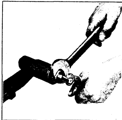
Fig. 24.—Removing Spring Eye Bushing with Puller 72355
