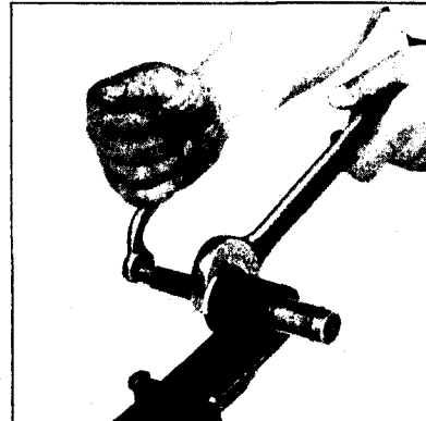
Fig. 25.—Installing Spring Eye Bushing with Puller 72355
