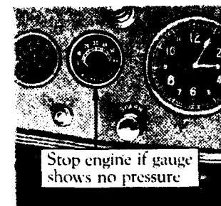
Fig. 8. The oil gauge does not indicate quantity; it only shows the pressure under which oil is forced to the engine bearings.
