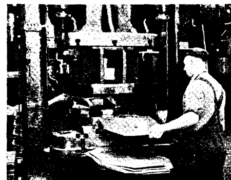
Oil pans, splash pans, and other sheet metal parts are stamped by giant presses to their correct form
