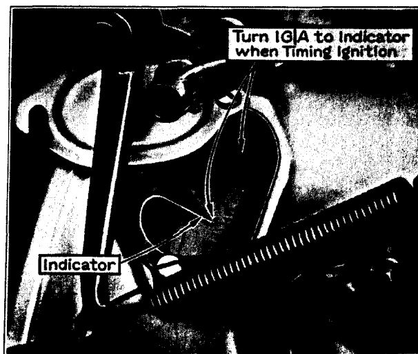
Fig. 21. The IG/A mark is 1\frac{1}{4} in. ahead of center.
