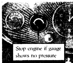
Fig. 7. The oil gauge does not indicate quantity; it only shows the pressure under which oil is forced to the engine bearings.
