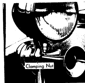
Fig. 39. The headlamps may be turned in any direction necessary for aiming after loosening the clamping nut at the base of the lamp.
