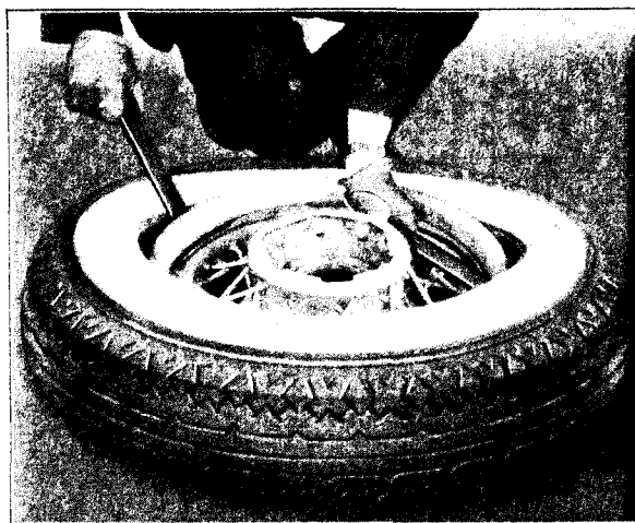
Fig. 105. Prying short lengths of the first tire bead over the rim flange
