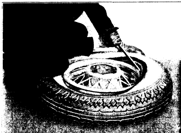
Fig. 108. Installing the second tire bead over the rim flange
