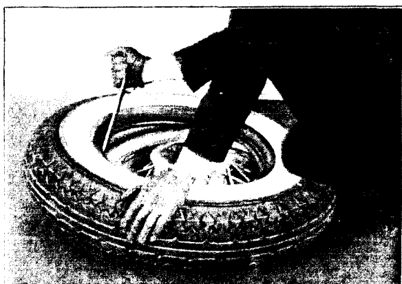
Fig. 107. Installing the first tire bead over the rim flange
