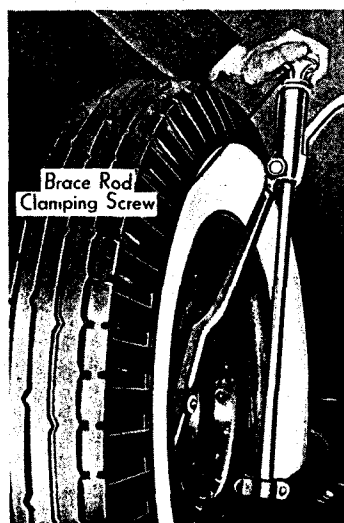
Fig. 33. The spare wheels on cars with fenderwell carriers may be removed after loosening the brace rod clamping screw.
