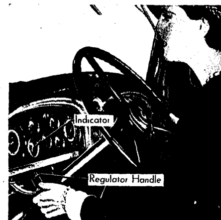
Fig. 12. The degree of ride regulation can be controlled by the handle on the left hand side of the steering column.
