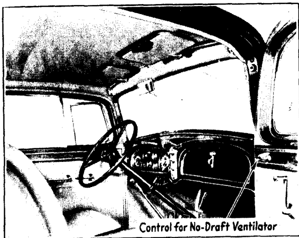
Fig. 2. Interior view of front compartment showing controls for door No-Draft ventilators
