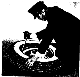
Fig. 34a. Coat both beads of the tire with vegetable oil soft soap before reinstalling the tire. Inflate the tube until barely rounded out and insert in the tire with the stem at the tire balancing mark. Place the tire on the rim, guiding the valve through the hole, and apply the rim nut loosely. Push the bottom bead down into the well at the valve and force the remaining portion of the bead over the rim flange, using a tire tool if necessary.
