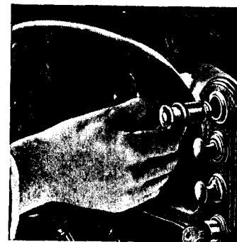
Fig. 19. To operate the cigar lighter press it in its socket, hold until the glow is seen; then remove it.
