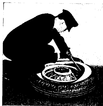
Fig. 34b. Force the top bead over the rim flange and into the well at the point opposite the valve. Kneeling on this side of the tire to hold it in the well, pry short lengths of the remaining portion of the bead, working around the rim until the entire bead is in place. Always keep as much of the top bead in the well as possible while prying the remainder of the bead.
