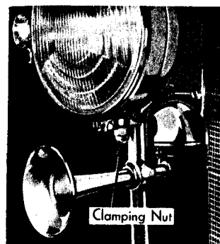
Fig. 38. The headlamps may be turned in any direction necessary for aiming after loosening the clamping nut at the base of the lamp.
