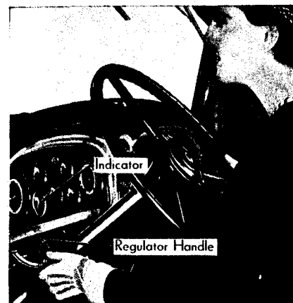
Fig. 12. The degree of ride regulation can be controlled by the handle on the left hand side of the steering column.
