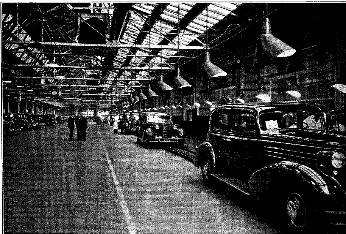
The La Salle moving down the final inspection line. At this point it has been road-tested and passed final inspection as to construction. When given the final o. k. by the inspectors as to equipment and finish, it is then sent to the loading dock for shipment
