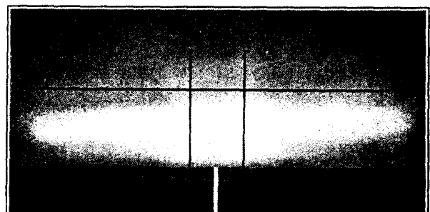
Fig. 51. Lower headlamp beam
