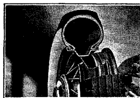
Drop Center Rim Construction
