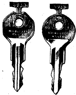
Fig. 11. The key numbers appear on metal tabs, which should be detached as soon as the car is received.
