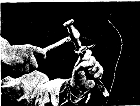
Illustration No. 100 Method of Cutting Roof Panel at Rear Quarter.
