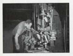
Balancing the crankshaft to 16 ounce inch limit, after which crankshaft, clutch and flywheel will be balanced within a 34 ounce inch limit. C
