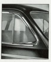
Roof mouldings and ventipane shields protect passengers from dripping water
