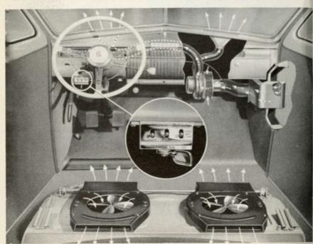
defroster with its own heating core, and fresh air inlet for ventilation, located under the instrument panel.
