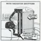
In Cadillac or LaSalle, water is free to flow from the radiator into the engine and back into the radiator at all times as soon as the engine starts. The shutters gradually open as the engine approaches normal operating temperature. When closed they prevent the flow of air through the radiator thus eliminating the need for anti-freeze in the cooling fluid while running.
