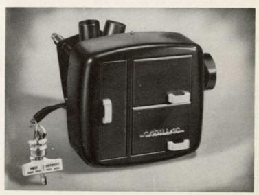
Direct and indirect heating is accomplished by utilizing a reversible motor. In direct heating, hot air is blown out of the face of the heater in the conventional manner, and normal defrosting is obtained. In indirect heating, the motor is reversed, and air is drawn in through the face of the heater and blown out the sides, top and bottom. In this position, the heat is diffused
