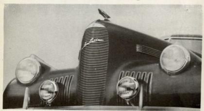
The Fog Lights are connected into the head lamp system of the car so that for maximum illumination under severe conditions, the head lights can be turned off. The tail lights and instrument board lights are turned on when the Fog Lights are on, regardless of the head lights being on, permitting operation of the car with the Fog Lights only.
