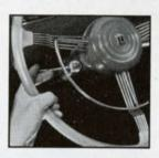
and right rear signals flash on and off for making a right turn. The left front and left rear signals flash for a left turn. Their extra brilliance and flashing feature make them easily distinguished at night above the continuous lighting system.
