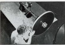
Accuracy of cam contours are carefully checked because of their importance to performance, with a micrometer and wheel graduated into minutes to simplify the reading of very slight irregularities on the cam surface.
