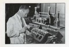
Cylinder bores are graded into one of 30 different sizes with a special expanding gauge.
