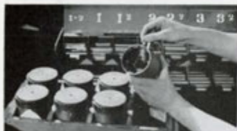
FITTING WRIST PINS BY HAND
