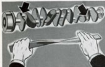
INERTIA FORCES ON STRAIGHT 8 CRANKSHAFT
