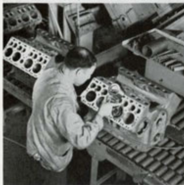
CHECKING CYLINDER WALL THICKNESS
