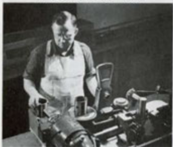
BEARINGIZING WRIST PIN HOLE
