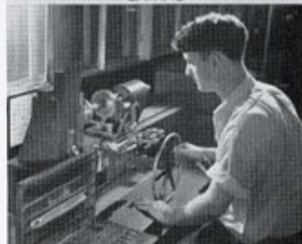
CHECKING HELIX ANGLE
