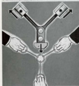
CANCELLATION OF INERTIA, 90° V-TYPE DESIGN
