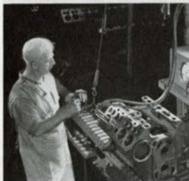
MEASURING BORES FOR SIZE
