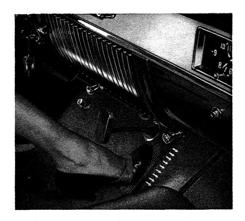
to the pressure exerted on the accelerator pedal and the speed of the car. Fourth gear, which is the normal running position after the car has gained momentum, has a ratio of 1 to 1. This results in exceptionally low engine speed compared to car speed, giving increased economy, smoother, quieter operation, lower oil consumption, and less wear on engine parts. This lower engine speed can make driving much more pleasing at higher car speeds.
