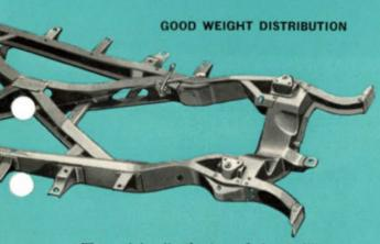
The weight distribution of the Cadillac car, approximately 50% on the front wheels and 50% on the rear, assures good traction for all four wheels. This means greater safety when rounding curves and surer, more positive braking. Contributing further to the road-hugging qualities of the 1956 Cadillac cars is the low center of gravity. It is a major factor in their amazing cornering ability and resistance to rollover.
