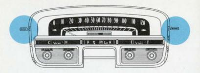
ment cluster. The left-hand lever marked "HEATER" turns the heater on and off and also controls the temperature. For most conditions, after the engine has warmed up (2 or 3 miles), push this lever down to the "LOW" position. If more heat is required, push the lever down farther.
