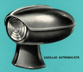
The Cadillac Autronic-Eye protects the Cadillac owner by causing the headlights of his car to switch to low beam when another car approaches from the opposite direction. Thus, the driver of the oncoming car is not blinded and both cars pass with greater safety. An overriding switch is provided to signal drivers who neglect to switch their own lights from bright to dim.
