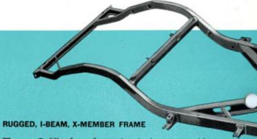
The new Cadillac frame for 1956, as in the past, provides the safety of sturdy, channel-section side rails with a rugged, I-beam, X-member extending beneath the entire passenger compartment. This type of construction, reserved for convertible models only by some car makers, provides a strong, rigid backbone for the entire car. The rugged front cross member provides sturdy support for the engine, steering and front suspension units.
