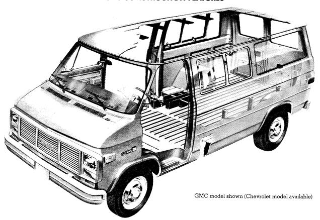
The all-steel, Chevy Van/Vandura and Sportvan/Rally bodies feature body-frame integral construction for outstanding structural rigidity and excellent durability. The basic bodies of either the nominal 15 foot (110" WB) or 17 foot (125" WB) models are comprised of an underbody structure, front end structure, left and right hand side panel structures, and a roof panel structure.
