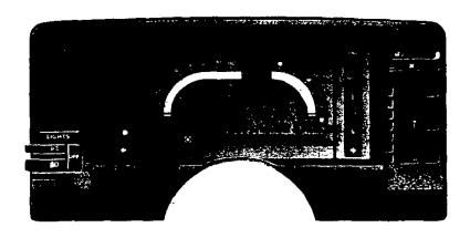
Standard Cluster with warning lights for engine temperature, generator, and oil pressure.
