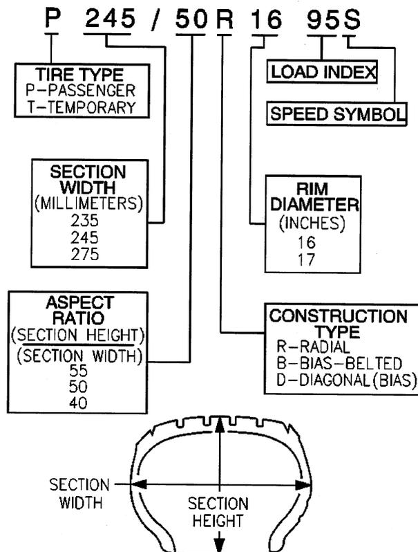
Most P-metric tire sizes do not have exact corresponding alphanumeric tire sizes. Replacement tires should be of the same tire performance criteria (TPC) specification number including the same size, the same load range, and the same construction as those originally installed on the vehicle. Consult a tire dealer if you must replace the P-metric tire with other sizes. Tire companies can best recommend the closest match of alphanumeric to P-metric sizes within their own tire lines.
