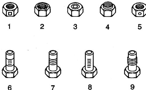
1. Prevailing Torque Nut, Center Lock Type
