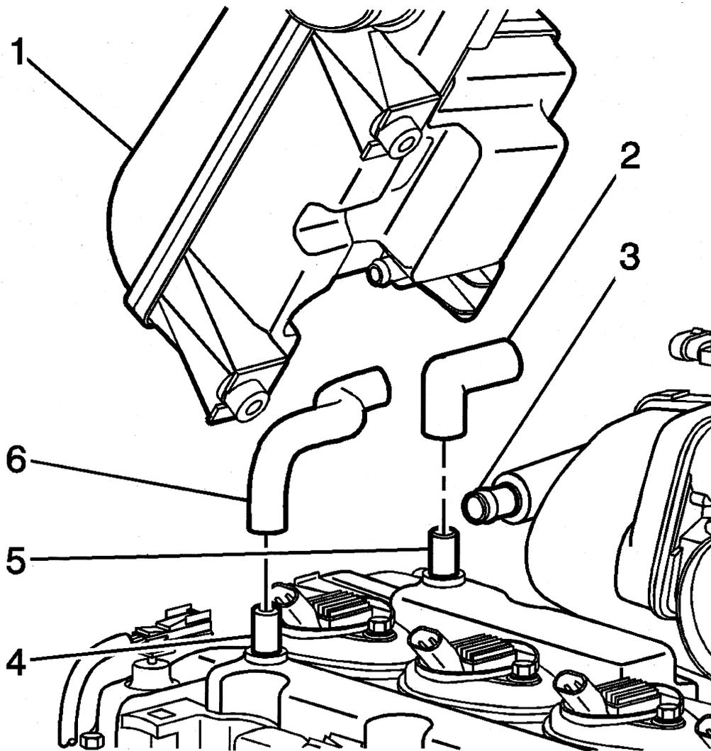
A crankcase ventilation system is used to consume crankcase vapors created during the combustion process instead of venting them to the atmosphere.
